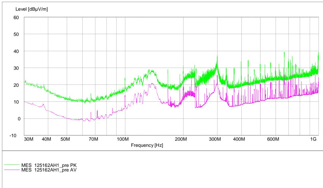
The following emissions were found during the preliminary measurement in this frequency range, so a final measurement was carried out on the open area test site. The results are presented in the following clause 5.3.2.2.
