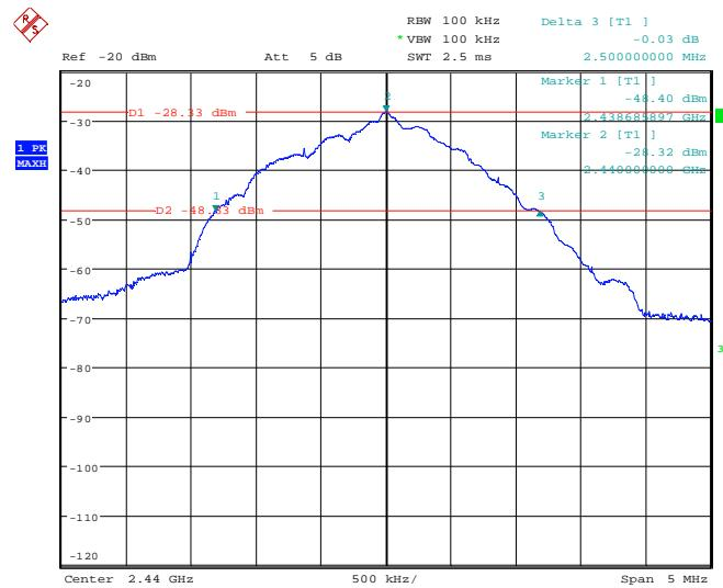
125162\_20dB\_low.wmf: 20 dB bandwidth of lowest channel (2481 MHz)
