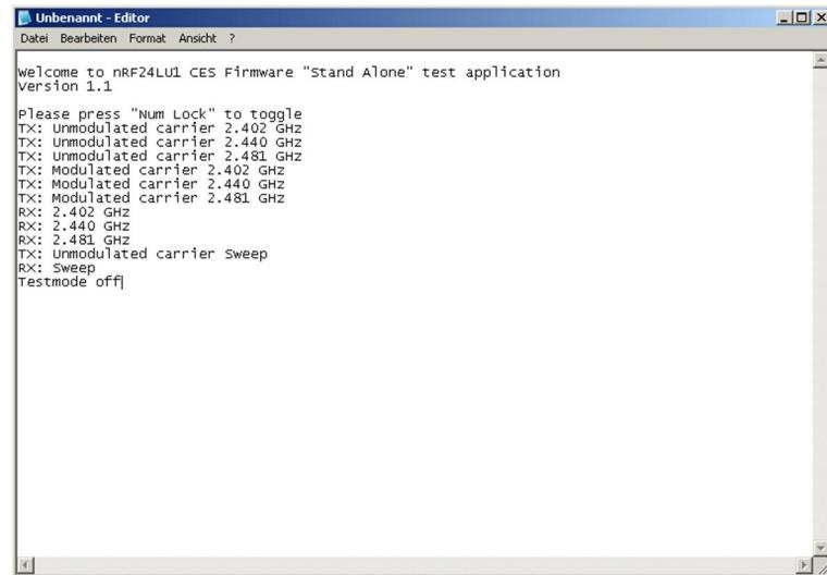
For the tests the continuous modulated transmission mode with maximum output power was used.
