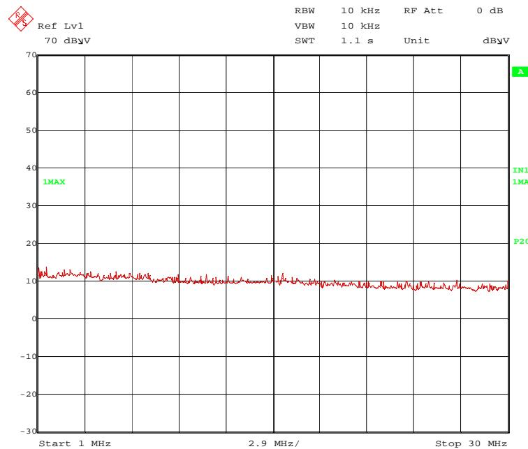
The emissions in the frequency range between 9 kHz and 1 MHz are caused by the ancillary notebook PC. From the EUT no significant frequencies above the noise floor of the system were found during the preliminary radiated emission test, so no measurements were carried out on the outdoor test site.
