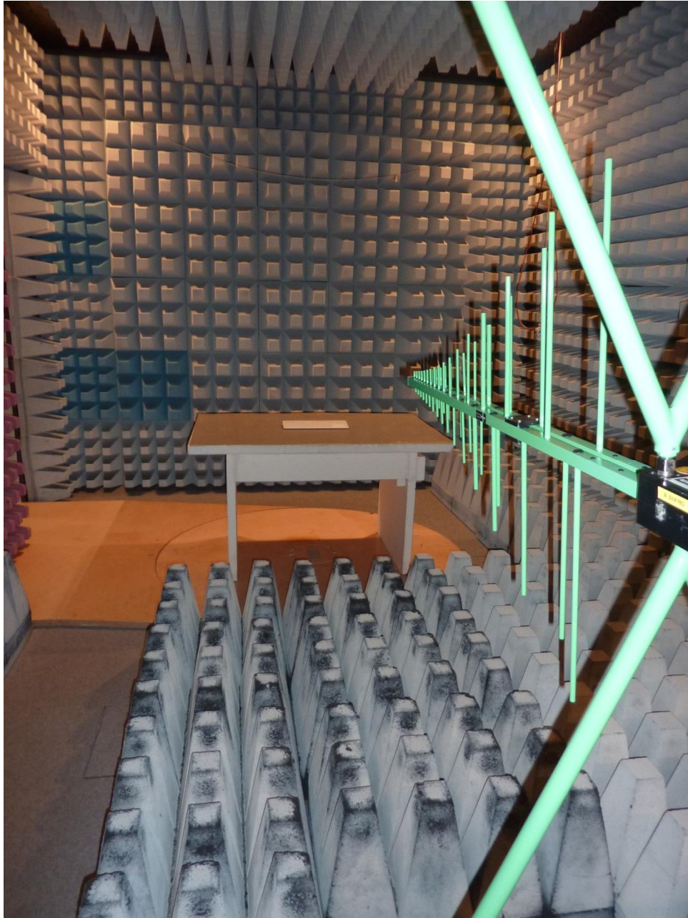
125162_2.JPG: Test setup fully anechoic chamber
