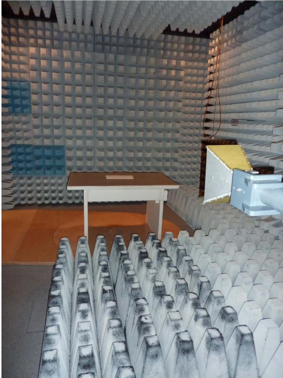
125162_3.JPG: Test setup fully anechoic chamber
