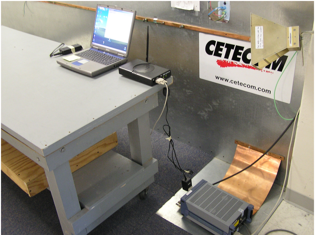
AC POWERLINE CONDUCTED EMISSIONS
