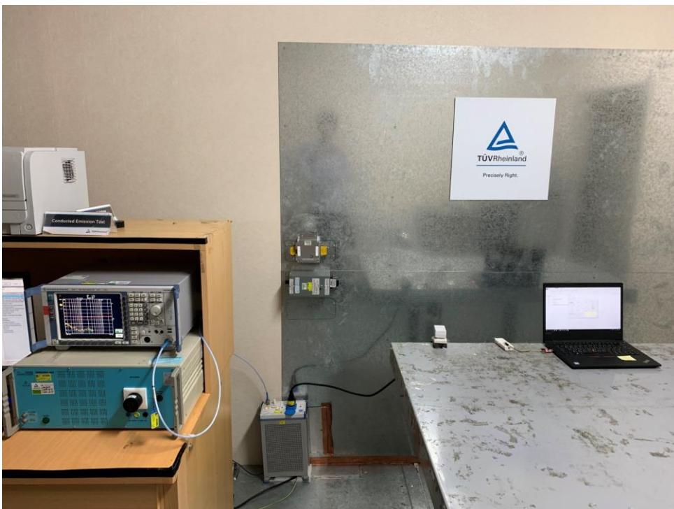
Photograph 8: Set-up for Mains Conducted testing (Front View)
