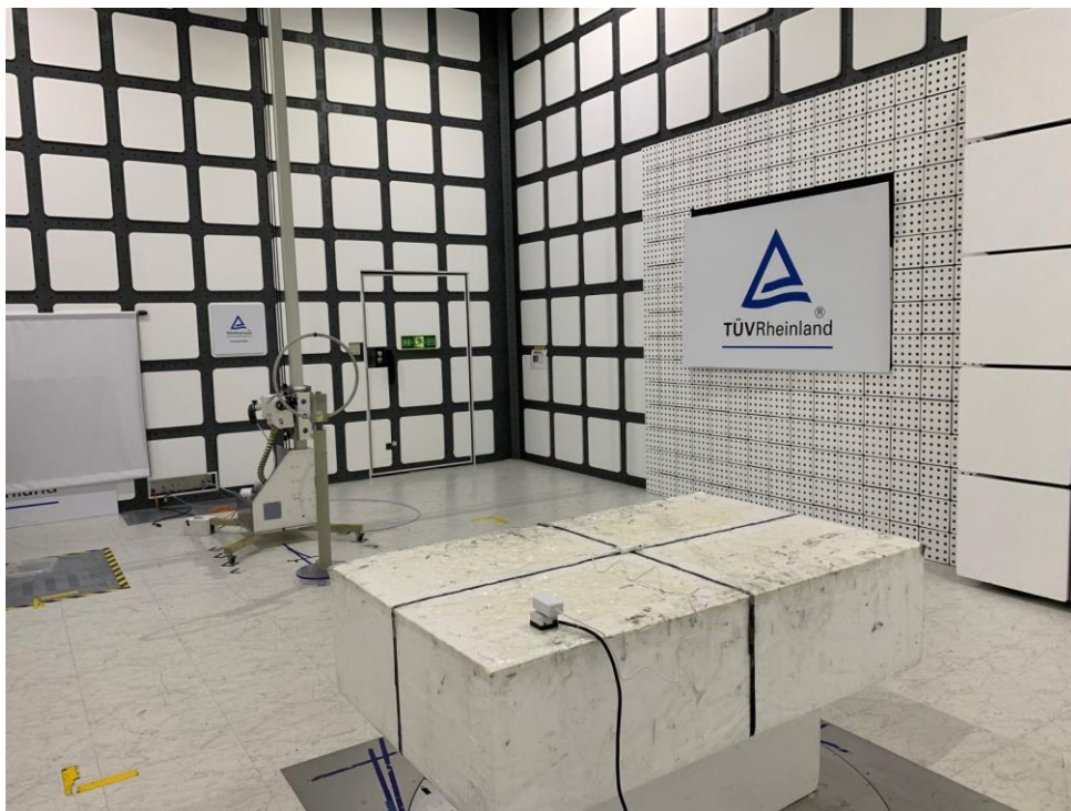
Photograph 4: Set-up for Spurious Emissions (Back View 3)
