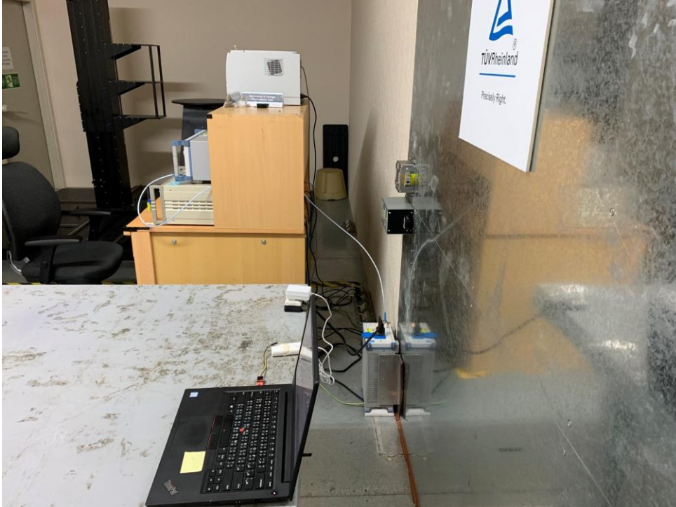
Photograph 7: Set-up for Mains Conducted testing (Back View)
