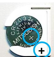
**Into the battery with + terminal facing down to battery holder.**
