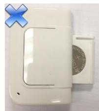
Positive battery terminal have to face down in battery holder.
