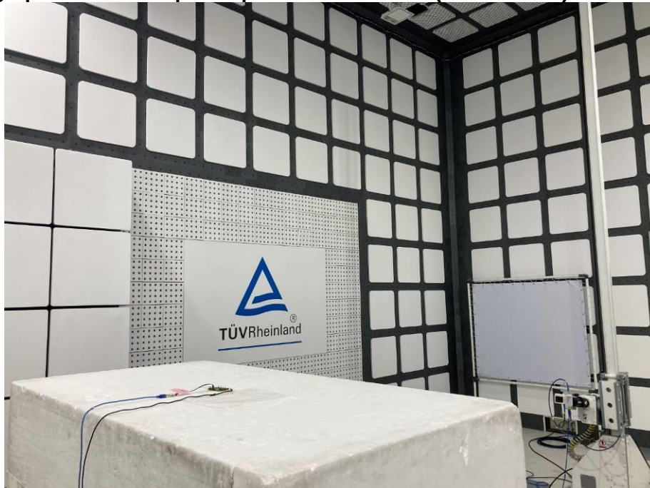
Photograph 6: Test Setup for Spurious Emissions (Back View 4)
