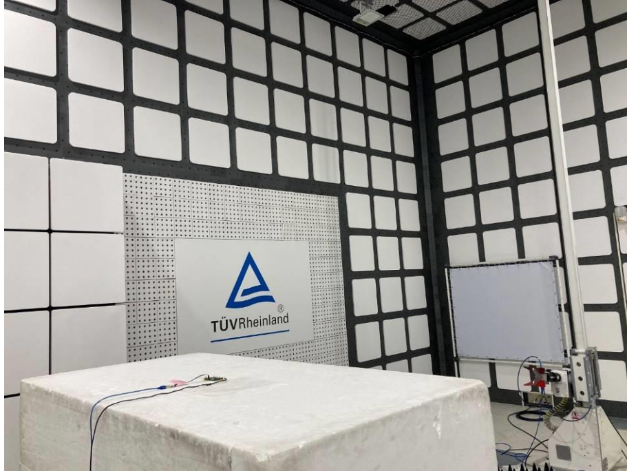
Photograph 6: Test Setup for Spurious Emissions (Back View 4)
