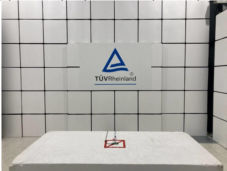
Photograph 1: Test Setup for Spurious Emissions (Front View 1)
