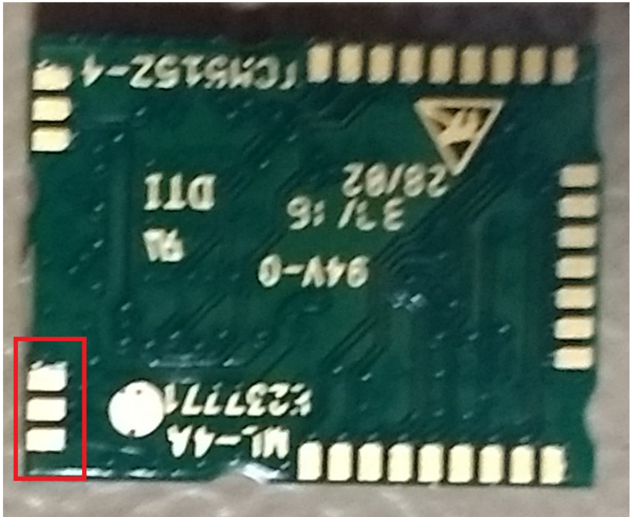
Figure 1: Bottom view of module: coplanar SMD pad antenna connector (red frame)
