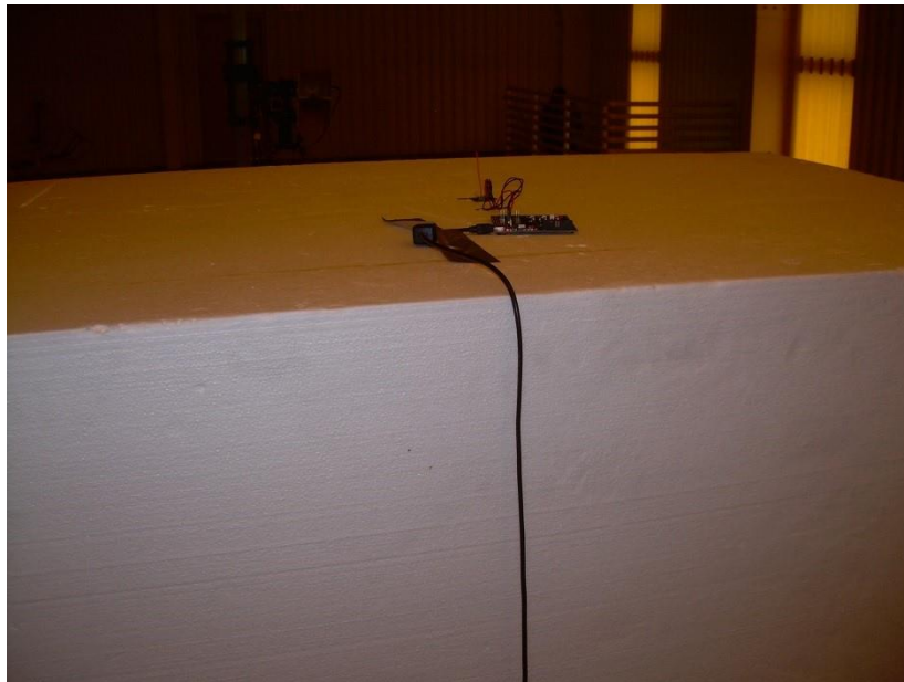
Photograph 4: Back View Radiated Emissions Configuration – Whip Antenna – Emissions Above 1000 MHz
