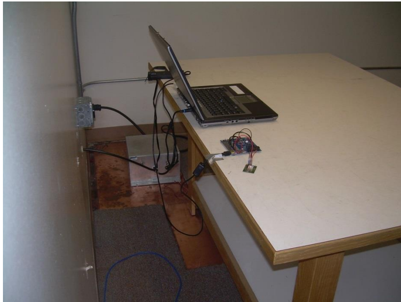
Photograph 10 - Back View Conducted Emissions Worst Case Configuration
