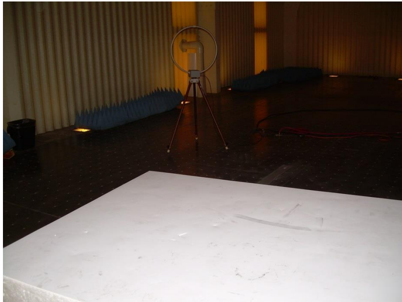
Photograph 24: Test Setup for Emissions Below 30 MHz
