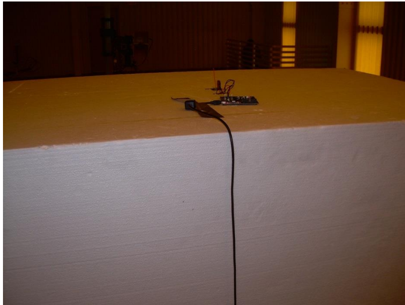
Photograph 4 – Back View Radiated Emissions Configuration – Whip Antenna – Emissions Above 1000
