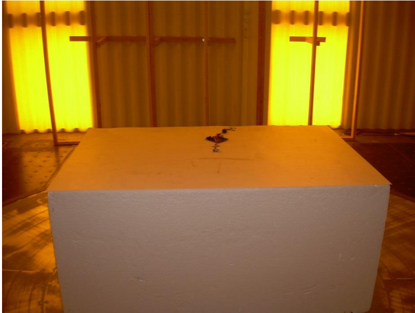
Photograph 1 – Front View Radiated Emissions Configuration – Whip Antenna – Emissions Below 1000 MHz
