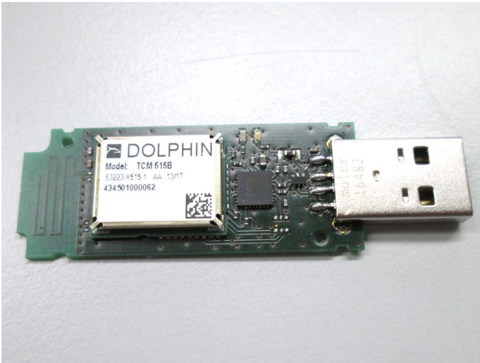
Photo A3-4: Demo-Board USB500Z-V1.0 with soldered EUT – Top view
