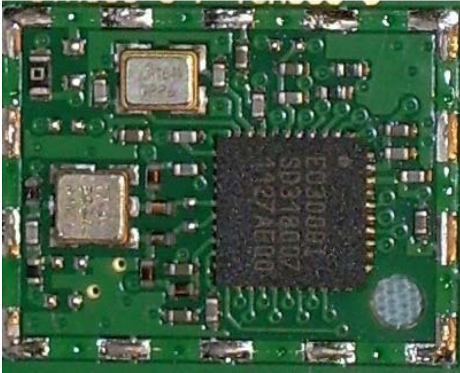
Photograph 8 – Circuitry Under RF Shield
