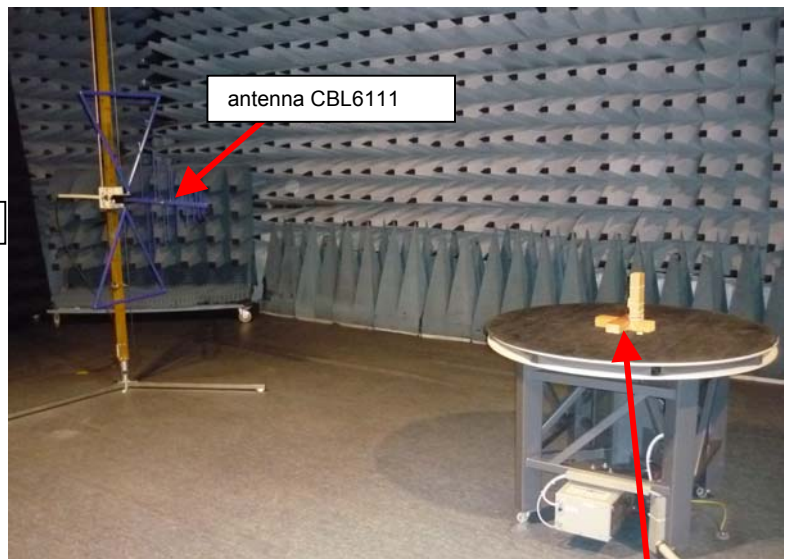
test setup for frequencies between 30MHz and 1000MHz
