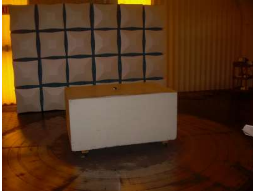
Photograph 1: Front View Radiated Emissions – Below 1000 MHz
