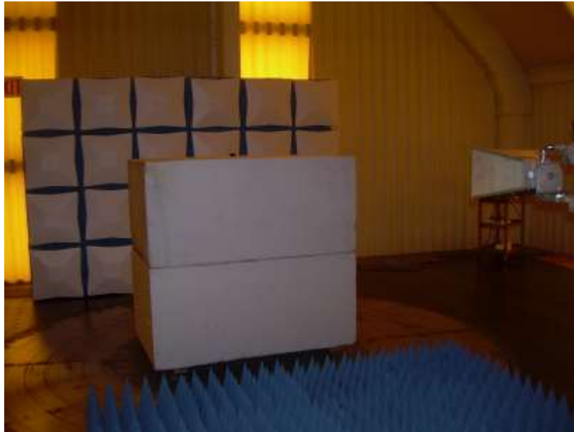
Photograph 3: Front View Radiated Emissions – Above 1000 MHz
