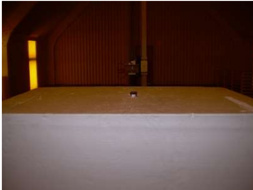
Photograph 4: Back View Radiated Emissions – Above 1000 MHz
