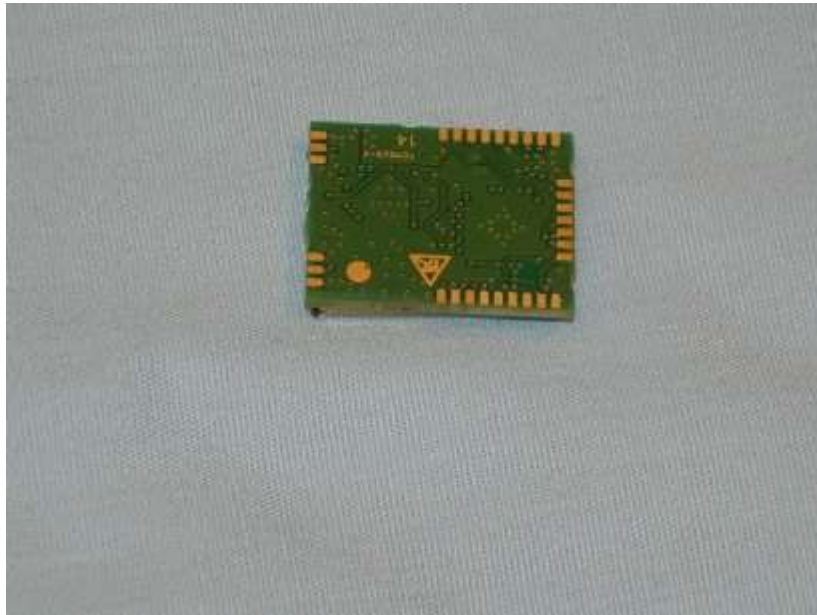
Photograph 18: Bottom Side of RF Module
