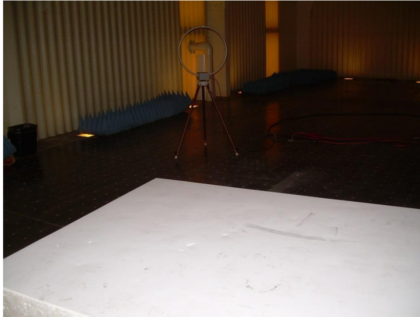
Photograph 13: Test Setup for Emissions Below 30 MHz
