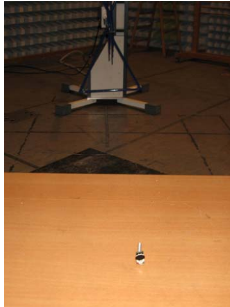
Figure 6-5: Test Configuration – Field Strength of Fundamental Wave
