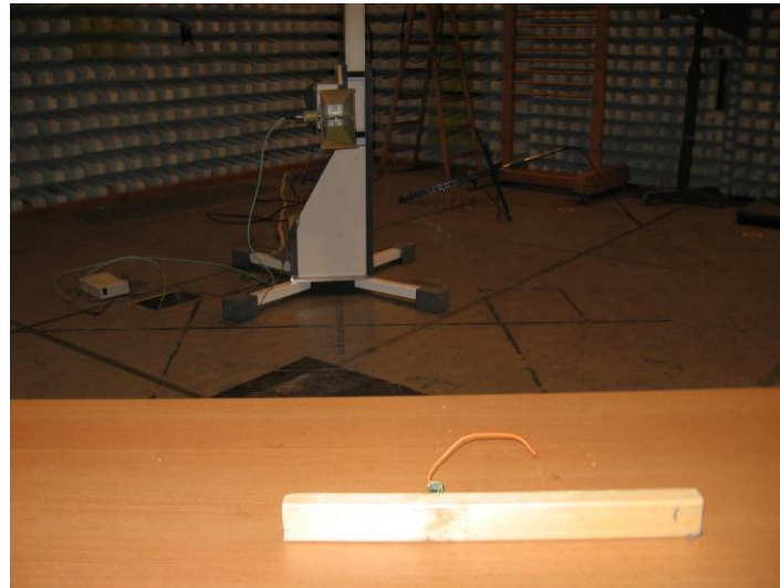
Figure 6-15: Test Configuration – Radiated Emissions (1GHz – 4GHz)
