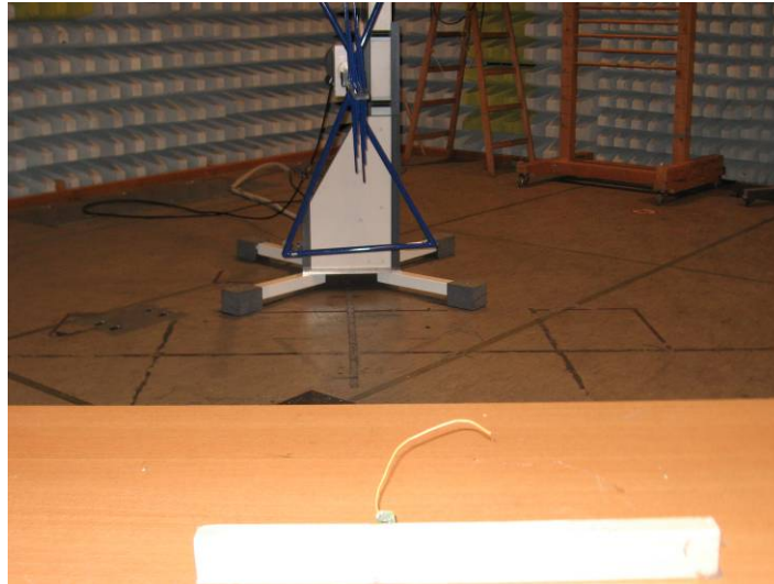
Figure 6-5: Test Configuration – Field Strength of Fundamental Wave
