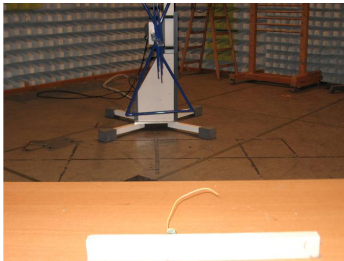
Figure 6-8: Test Configuration – Radiated Emissions (30MHz – 1GHz)
