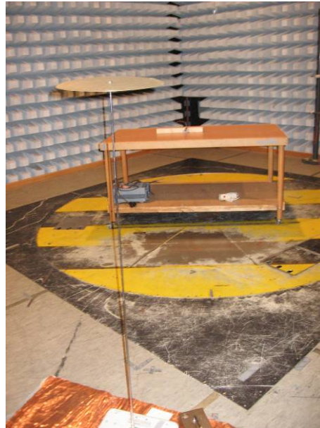
Figure 6-6: Test Configuration – Radiated Emissions (9kHz – 30MHz)
