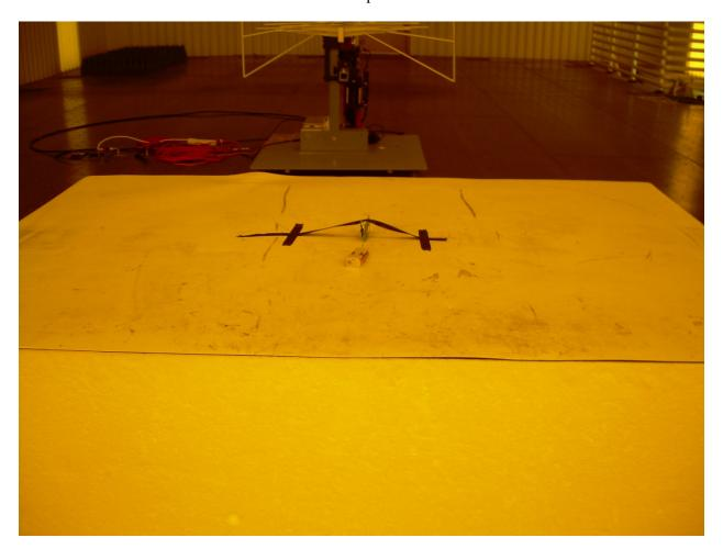
Front View Radiated Disturbance – On Edge Configuration
