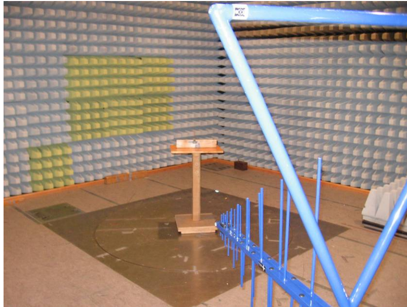
Figure 6-4: Test Configuration – Field Strength of Fundamental Wave
