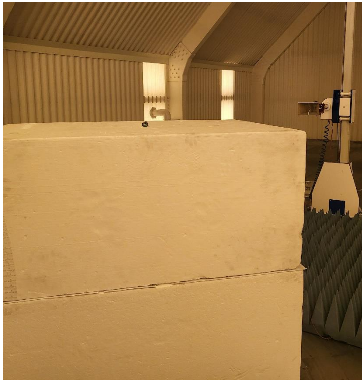
Photograph 4: Back View Radiated Emissions Worst Case – Above 1000 MHz Configuration
