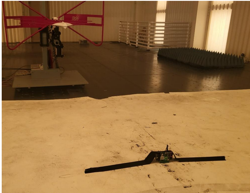
Photograph 2: Back View Radiated Emissions, Below 1000 MHz Worst Case Configuration
