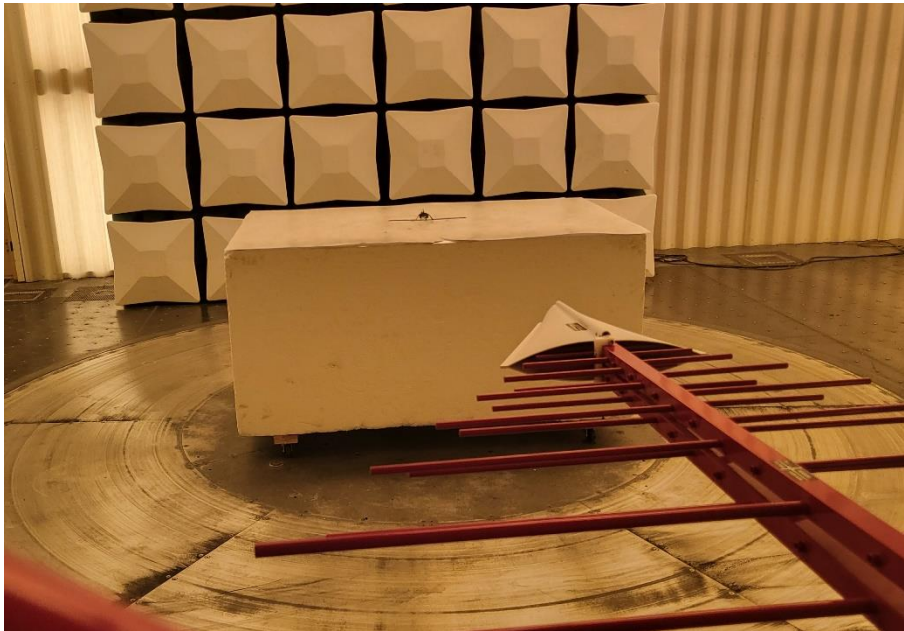
Photograph 1: Front View Radiated Emissions, Below 1000 MHz Worst Case Configuration
