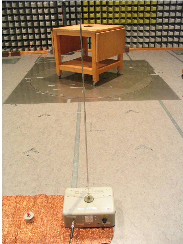
Figure 6-8: Test Configuration – Radiated Emissions (9kHz – 30MHz)
