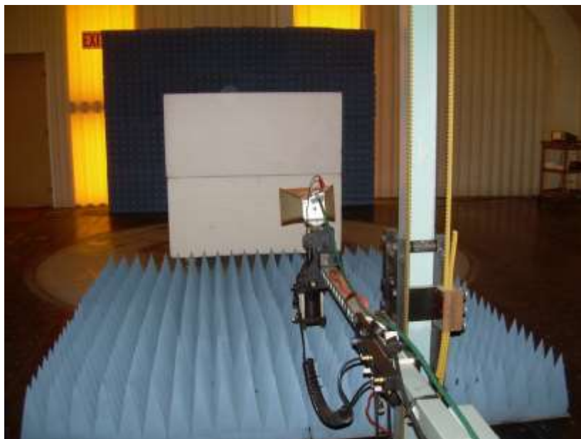
Photograph 10: Reference Photo of Test Setup for Emissions Above 1000 MHz
