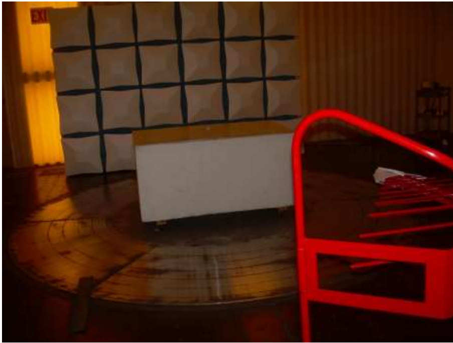
Photograph 1: Front View Radiated Emissions, Below 1000 MHz Worst Case Configuration
