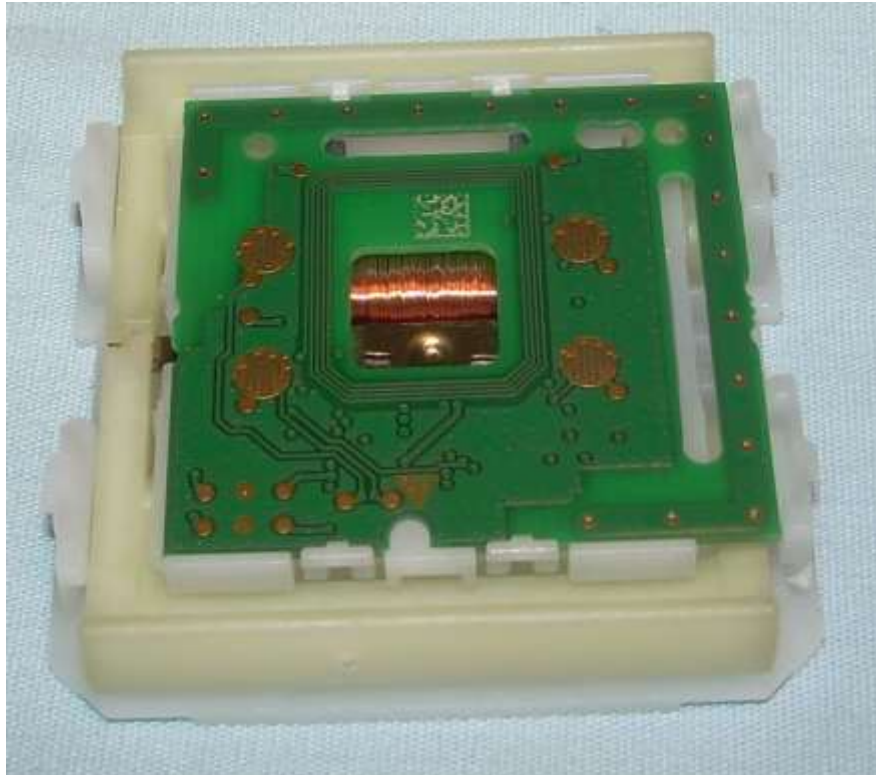
Photograph 5 – PCB Placement Inside EUT
