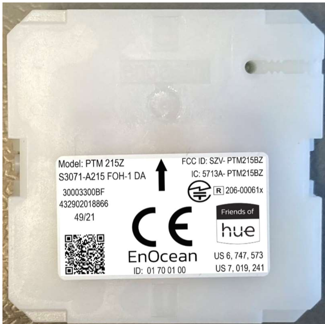
Figure 1 Label Placement PTM 215Z FOH
