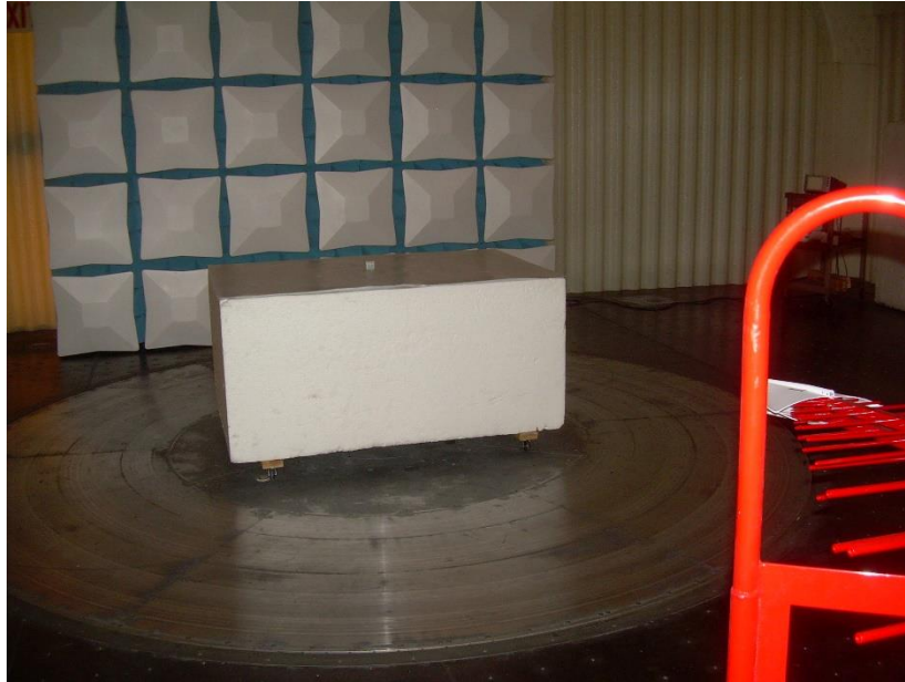
Photograph 1: Front View Radiated Emissions Configuration – 30 to 1000 MHz
