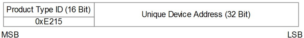
Figure 11 – BLE static source address structure
