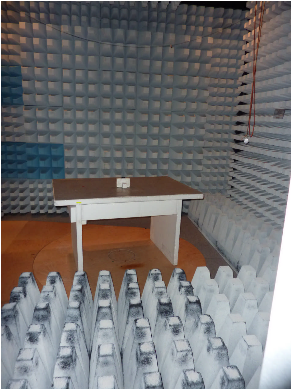
112808_c.JPG: PTM210 C, test setup fully anechoic chamber
