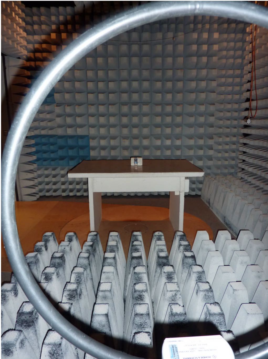
112808_d.JPG: PTM210 C, test setup fully anechoic chamber
