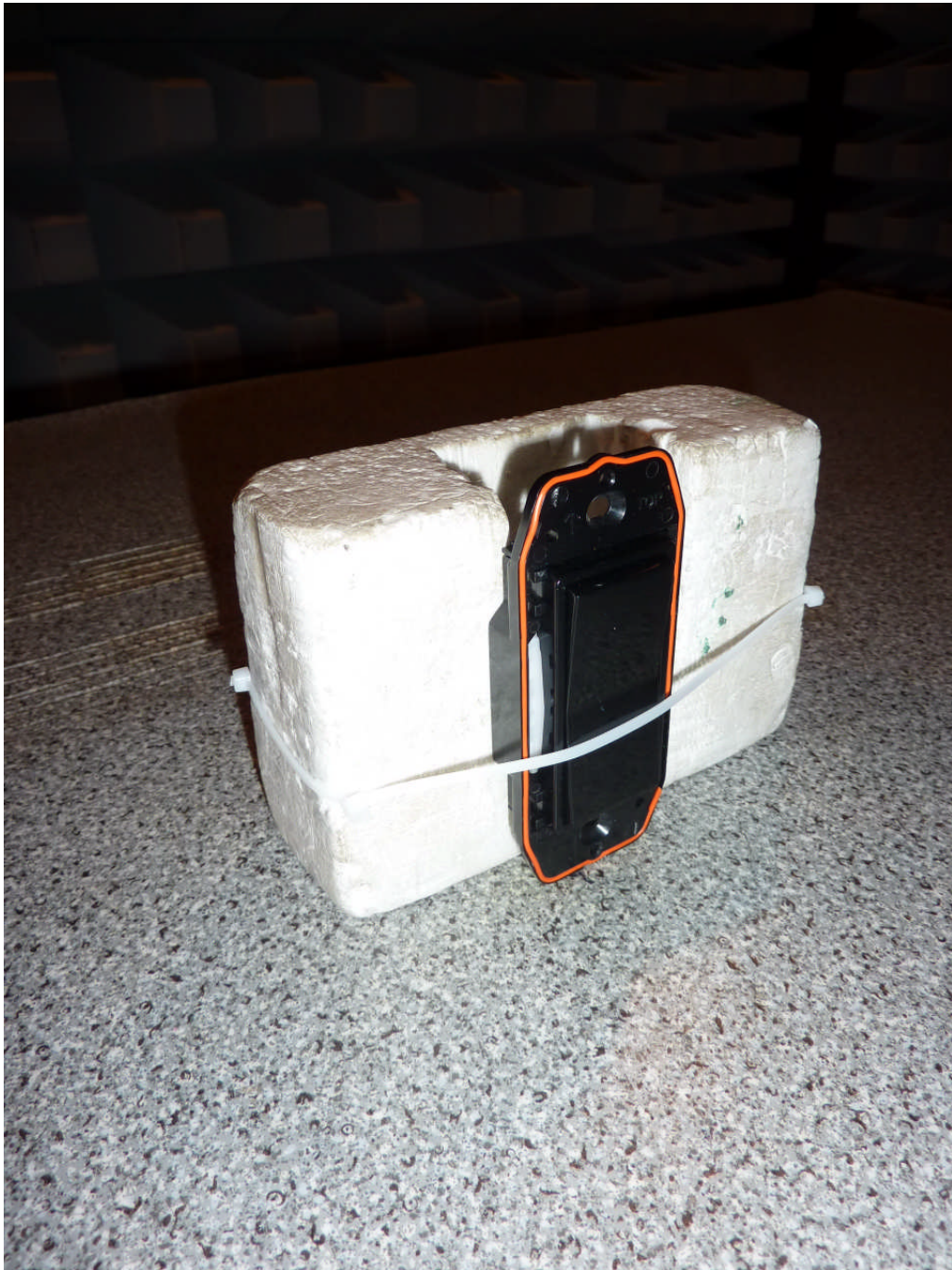
112808_b.JPG: PTM210 C, test setup fully anechoic chamber
