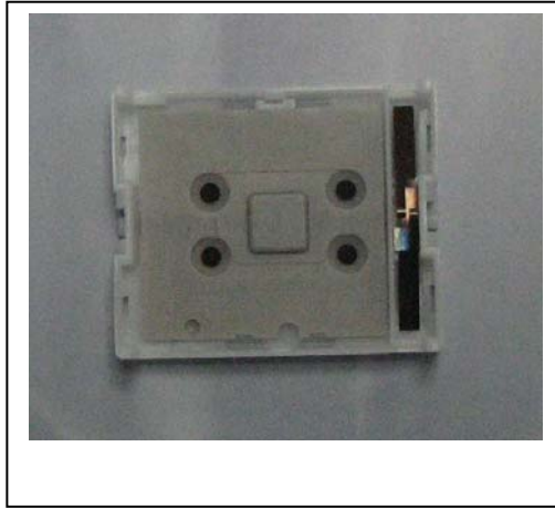
Fig. 2: Top Case including contact mat and flatspring
