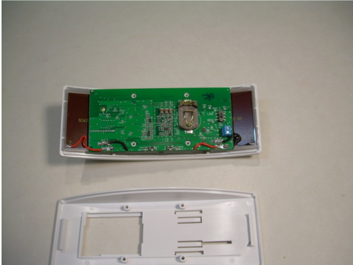
Photograph 5 – View of the EUT and back of PCB with Back Cover Removed
