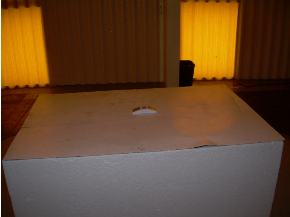
Photograph 1 – Front View Radiated Disturbance Worst Case Configuration
