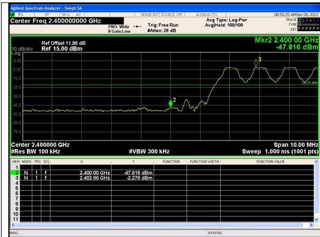
Out Of Band Emission(Left) GFSK_DH5_Channel Hopping
