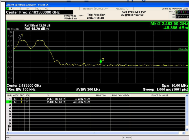
Out Of Band Emission(Right) GFSK_DH5_Channel Hopping
