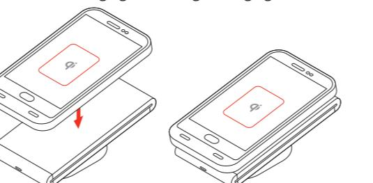
**4** While in standby mode, the LED is OFF. When the device is first placed on the pad, the LED blinks 3x indicating a wireless connection has been made. When power transfer begins the LED will turn solid. At the end of charge the LED will turn off.
