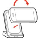
While in Standby mode, the LED is OFF. Solid red LED indicates Verizon Qi Wireless Charging Stand is delivering full power. LED indicator light
