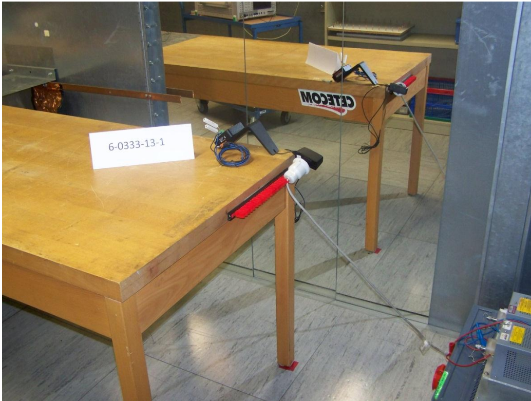
Photograph 1: Measurements of conducted emissions on AC-mains
