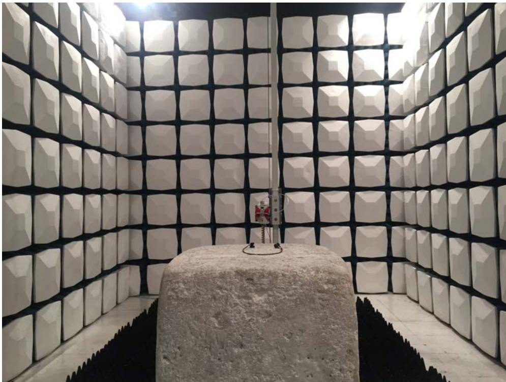
Description: Radiated Emission Test Setup for 1~18GHz
