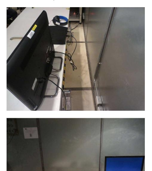
Test Setup Photo - Conducted Emission
