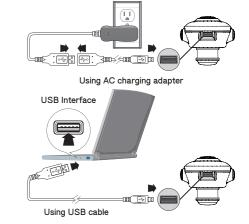
(1) Be sure the USB connector is aligned correctly and do not force the connection. Use the USB icon on the connector and in the illustrations below as a guide.
