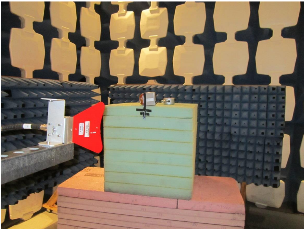
Radiated Emissions - 6 to 18 GHz
