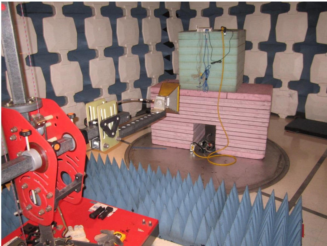
6GHz – 18GHz (worst case orientation)
