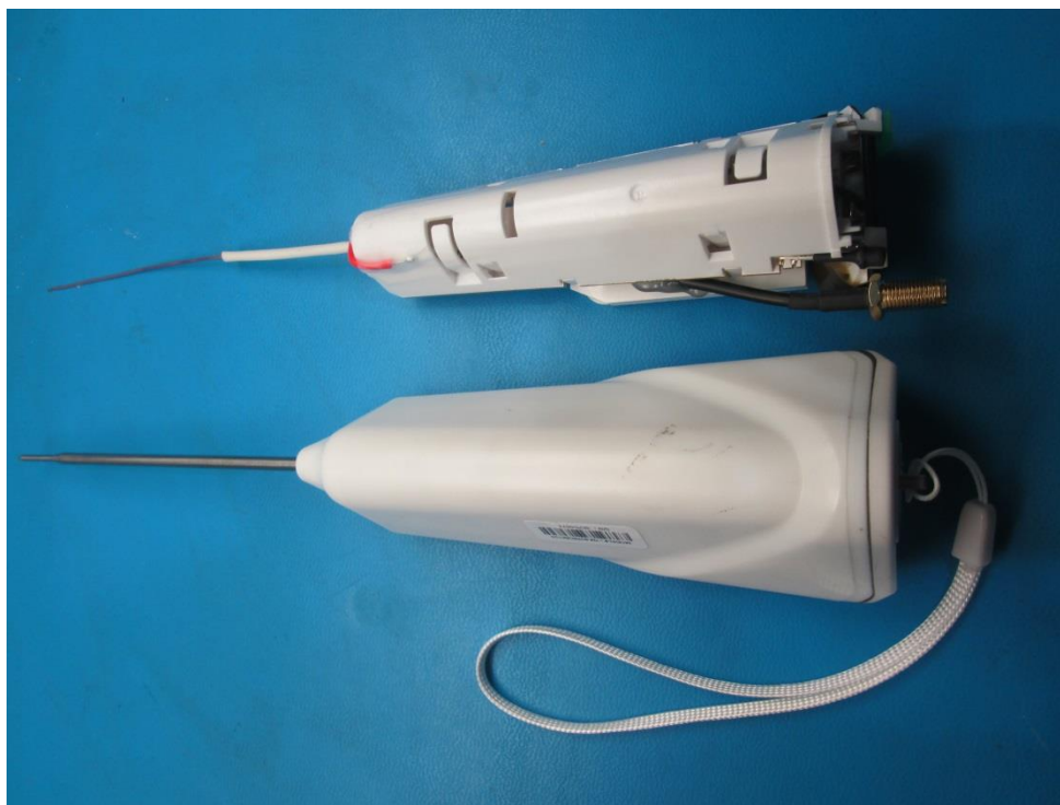
Bluetooth LE Kitchen Thermometer, Bottom View, SMA Coupler for Testing Only
