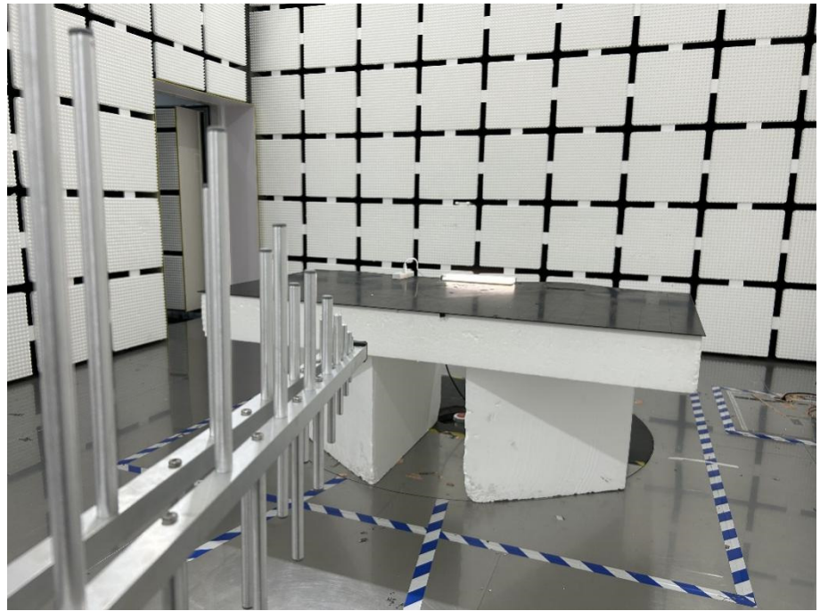
Radiation Emission Test Setup (30MHz to 1GHz)
