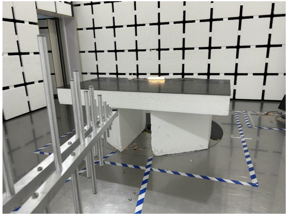
Radiation Emission Test Setup (30MHz to 1GHz)
