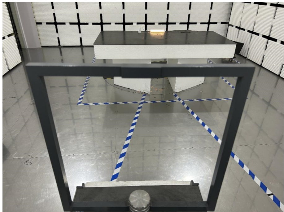
Radiation Emission Test Setup (Below 30MHz)
