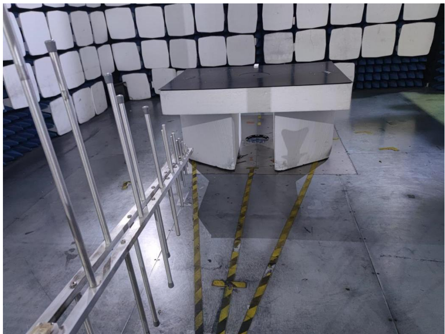
Radiation Emission Test Setup (30MHz to 1GHz)
