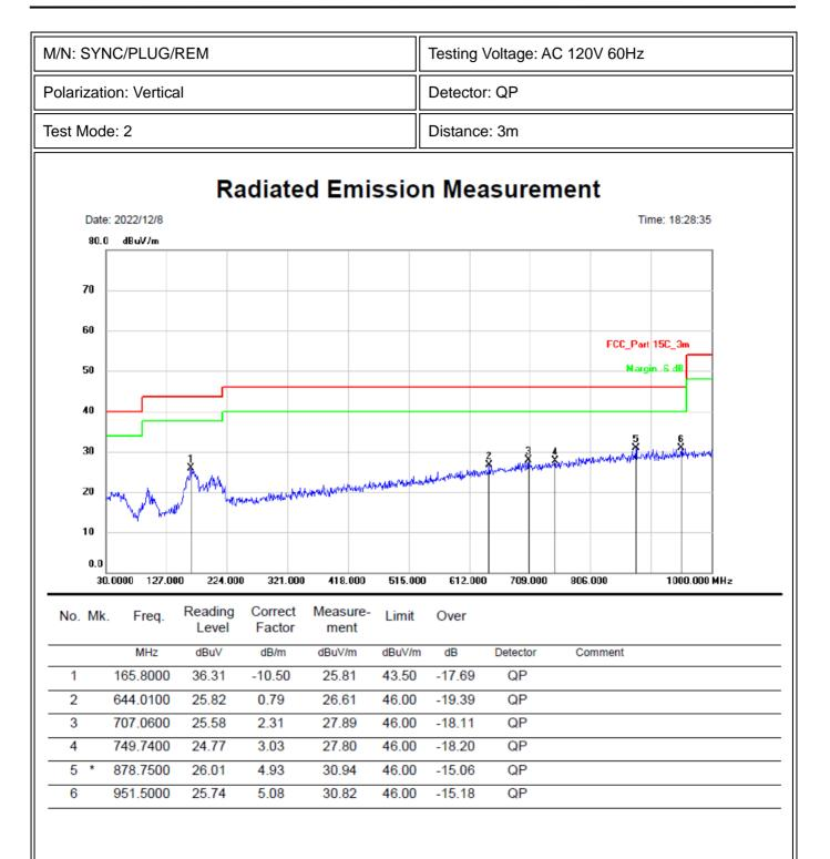
Note: Below 30MHz, the emissions are lower than 20dB below the allowable limit.
