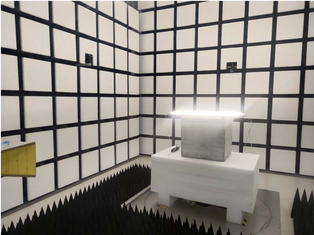
Radiated Emission Above 1GHz View
