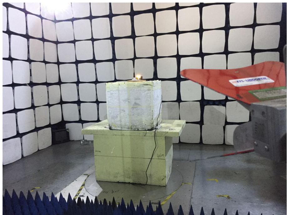
Radiation Emission Test Setup (1GHz to 18GHz)
