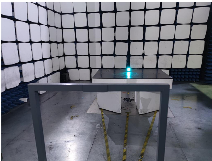
Radiation Emission Test Setup (Below 30MHz)
