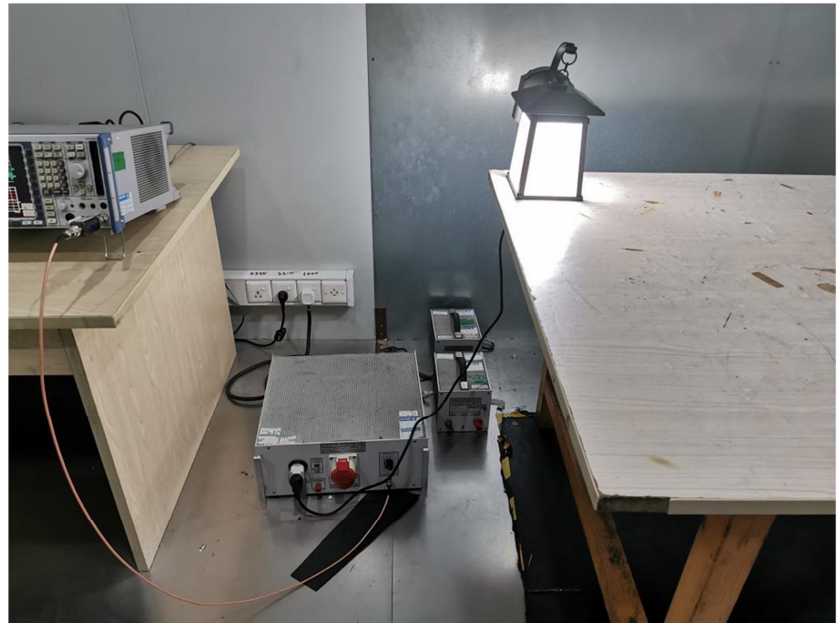
Conducted Emission Test Setup
