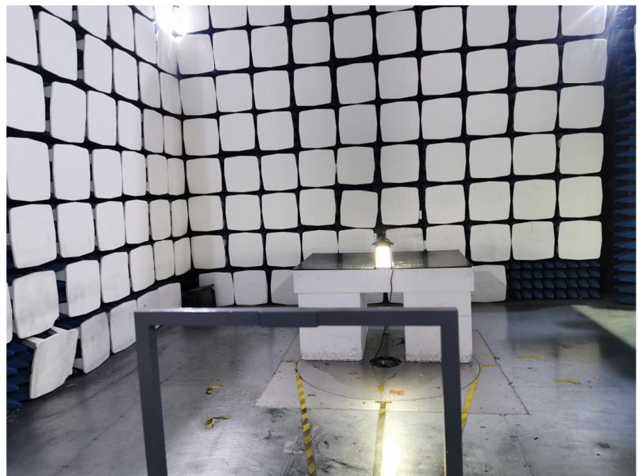
Radiation Emission Test Setup (Below 30MHz)
