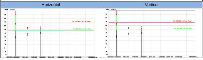
Remark: The emissions for frequency above 18GHz are attenuated 20dB below the limit, it does not record in report.
