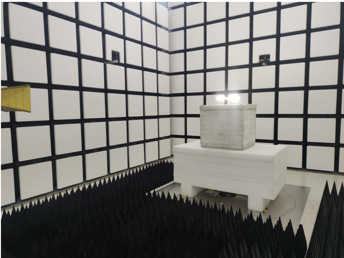
Radiated Emission Above 1GHz View
