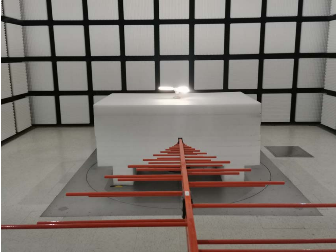
Radiated Emission Above 1GHz View
