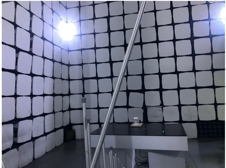
Radiation Emission Test Setup (30MHz to 1GHz)
