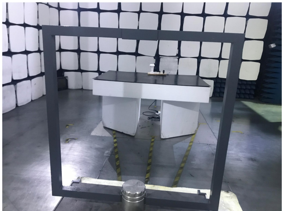
Radiation Emission Test Setup (Below 30MHz)
