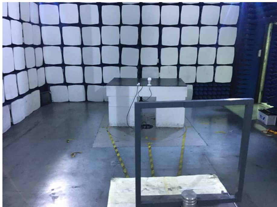
Radiation Emission Test Setup (Below 30MHz)
