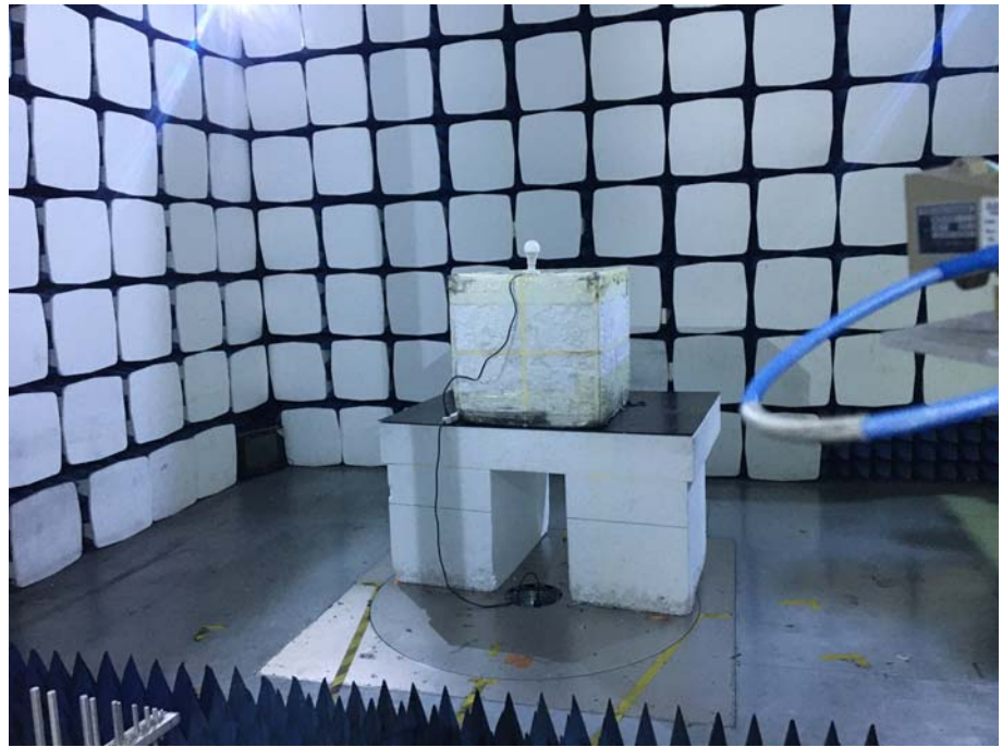
Radiation Emission Test Setup (Above 18GHz)
