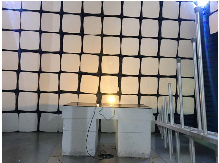
Radiation Emission Test Setup (30MHz to 1GHz)
